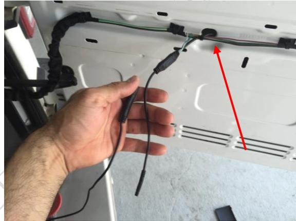
6. Pass the camera wiring from the outside of the gate into the inside using pre-existing wiring holes.
