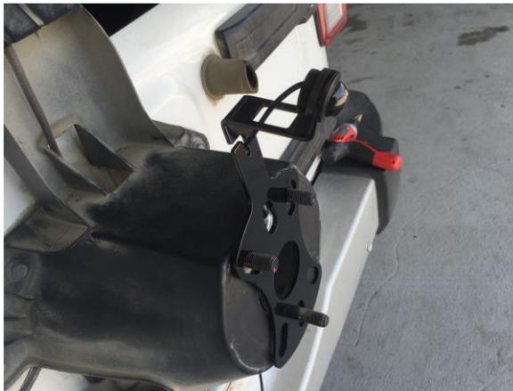
4. The Wrangler Lockpick Camera can now slide over the studs in the tire mount.
