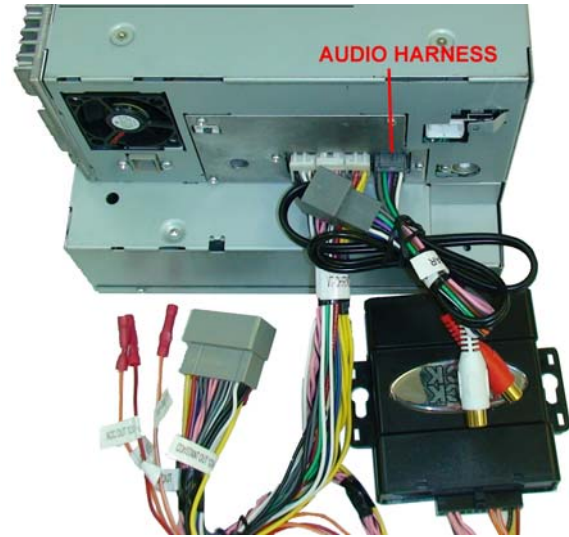
IF YOU DO NOT HAVE FACTORY VES, PLUG IN THE VES AUDIO CONNECTOR.
