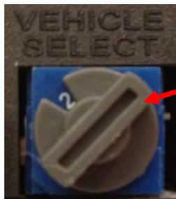
Place rotary switch on number 2 position and all communication switches **UP** as shown in the photos here.
