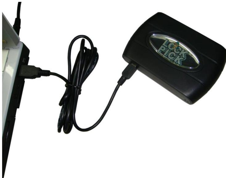
(make sure module is also connected to Lockpick harness and vehicle)
