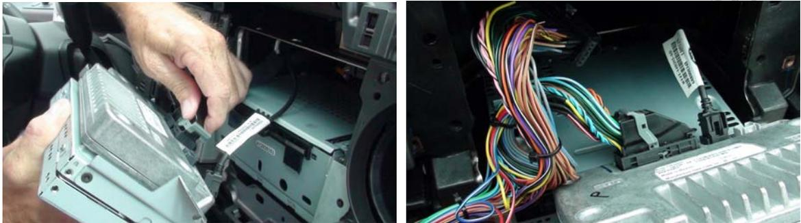
The Lockpick harness is simple to install and consists of matching male and female connectors which are installed in-line with the original factory connection. Plug the factory connector removed earlier into the matching female Lockpick connector. Finish by plugging the male Lockpick harness connector back into the previous factory location.
