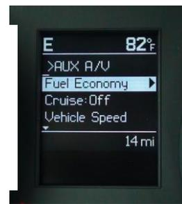
When the AUX A/V function is selected, the Lockpick will enter into a sub menu and display >AUX A/V V This indicates that the AUX A/V function is now selected (>) and the Video (V) is active and displaying the picture from the source connected to the Video 2 input on the Lockpick module. You may toggle the Video (V) OFF and listen only to the audio by pressing the BACK button on the steering wheel 2x. Press the Back button 2x again and the Video (V) will toggle back ON.
