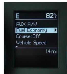
**Fact AUX** – Within your console are inputs for an additional audio input. To activate and listen to a device connected to the factory Aux input, select the Fact AUX Lockpick menu. Note: If audio is input to the Lockpick AUX A/V input and the factory Aux input at the same time, mixing of audio will occur. To prevent this, only use one at a time.
